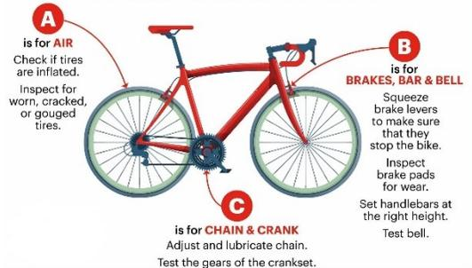
If any of these things are not working correctly, visit a local bicycle shop to have repairs made.
